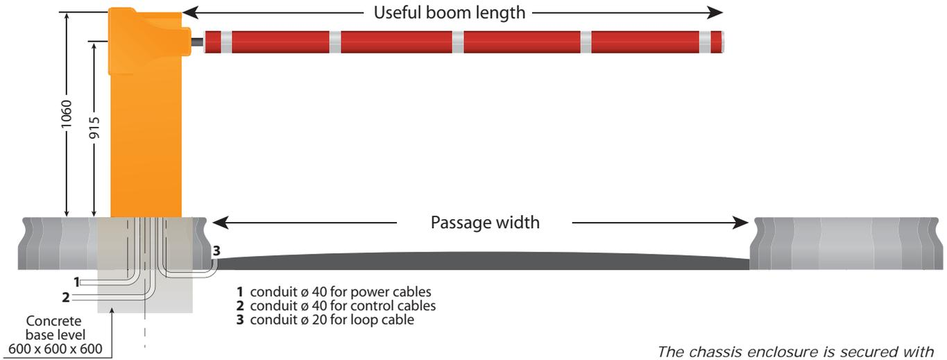
The chassis enclosure is secured with 4 screws and 4 washers. It is possible to fix the barrier with M12 chemical anchors
