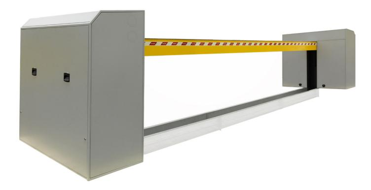
Motorized barriers with vertical movement, called **BL M50 LIFT BARRIER**, have a considerable mechanical strength to meet the highest anti-terrorism security because they are designed to resist to a breakout of a truck having a weight of 6.800kg which impacts at 80km/h (according to legislation uSA SD-STD-02.01 - today ASTM F2656-07).
