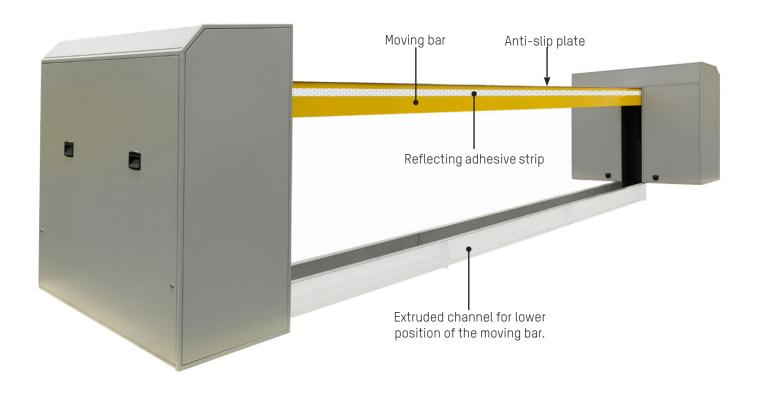
The motorized barriers with vertical movement, called **BL M50**, have a considerable mechanical strength to meet the highest anti-terrorism security resquests because they are designed to resist to the breakout of a truck having a weight of 7.500kg which impacts at 80km/h (See also the technical caracteristics).
